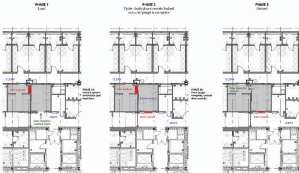
Figure 1: The sequencing of the decontamination process through each of the three phases.
